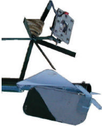
Fig. 6 - The camera housing attached to the chassis.
