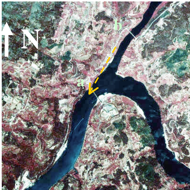
Fig. 1 - Air photo of the junction of rivers Douro and Tamega. Douro flows from East to West, whereas Tamega comes from Northeast with an alignment closely incident on the fallen P4 pillar. Also seen bridges a) Hintze Ribeiro – Douro - and b) Duarte Pacheco - Tamega. Photo width is approximately 3,5km.
