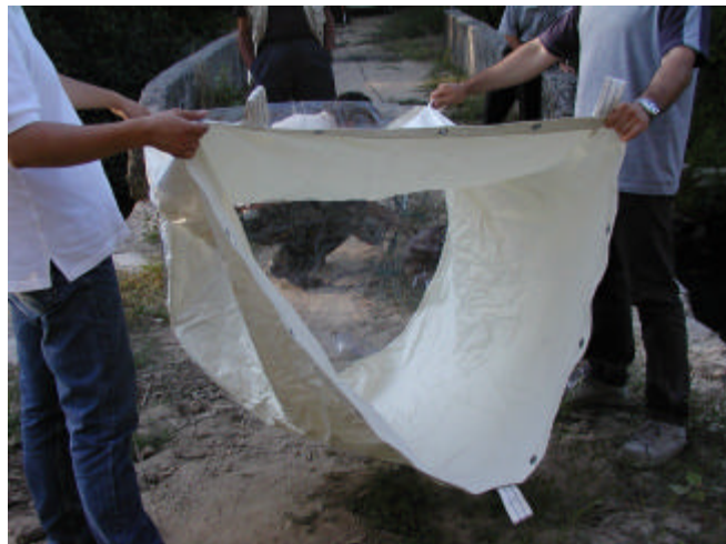
Fig. 3 - Canvas bubble with transparent flexible window.
