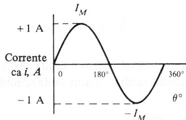
$$\text{Se: } v = V_M \text{sen}(\omega t + \theta) \Rightarrow i = I_M \text{sen}(\omega t + \theta) = \frac{V_M}{R} \text{sen}(\omega t + \theta)$$
