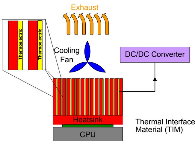
Fig. 3: Illustration of the CPU passive heat sink cooling apparatus and active air exhausting system with the thermoelectric scavenging devices connecting to the step-up converter stage.
