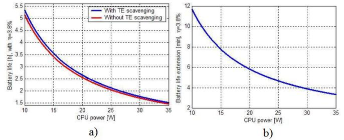
Fig. 11: Battery extension analysis at 3.8% efficiency obtained for a temperature gradient of 75 °C.
