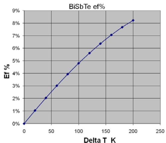
Fig. 1: Thermoelectric BiSbTe efficiency vs differential temperature.
