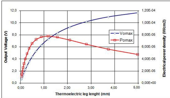
Fig. 9: Open-circuit output voltage and power of a  $1 \text{ cm}^2$   $\text{Bi}_2\text{Te}_3$ - $\text{Sb}_2\text{Te}_3$  thermoelectric generator, plotted as function of the leg length.
