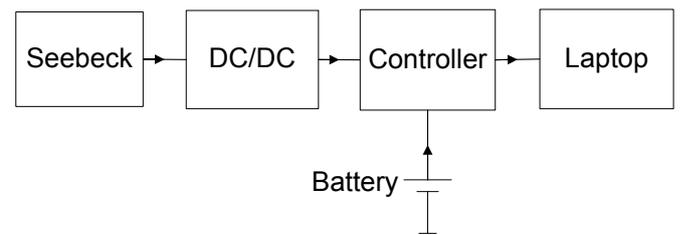
Fig. 3: Block diagram of the system architecture.
