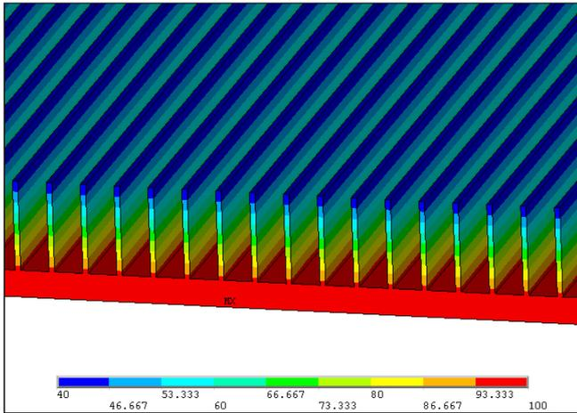
Fig. 2: Illustration of the temperature gradient across the heatsink using a FEM tool.
