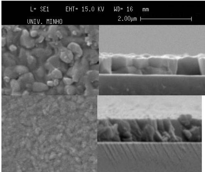
Fig. 4: SEM top view (left) and cross-sectional (right) images of Bi<sub>2</sub>Te<sub>3</sub> (top) Sb<sub>2</sub>Te<sub>3</sub> (bottom) thin-films.
