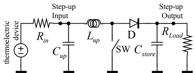
Fig. 7: Schematic of a simple step-up circuit.
