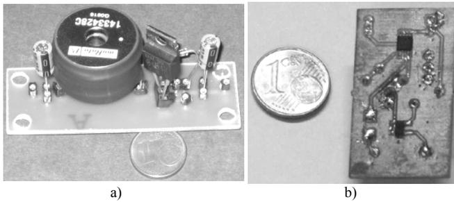
Fig. 8: Photographs of a) a prototype of the simple step-up converter, and b) of the charge-pump, followed by the step-up.
