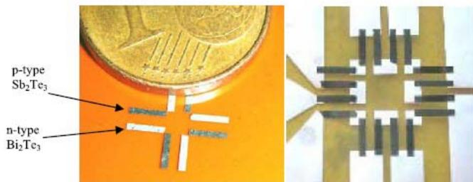
Fig. 5: Photograph of n-type and p-type elements, before deposition of top contacts (left), and a photograph of a thermoelectric micro converter with eight pairs of thermoelectric elements, fabricated with bottom contacts (right).
