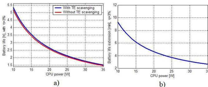
Fig. 10: Battery extension analysis at 3% efficiency obtained for a temperature gradient of 60 °C.
