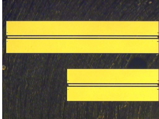
Figure 4. Sample of the fabricated coplanar waveguides used for S-parameter measurement.
