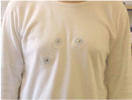
Figure 6. A photo of the patient wearing a electronic shirt ready to plug the RF sensing module (antenna + transceiver). We can see the three connections for heart-rate with a single electrode, respiratory function and posture.
