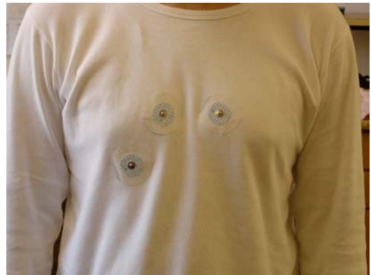
Fig. 5. A photo of the patient wearing a electronic shirt ready to plug the RF microsystem (antenna + transceiver). We can see the three connections for heart-rate with a single electrode, respiratory function and posture
