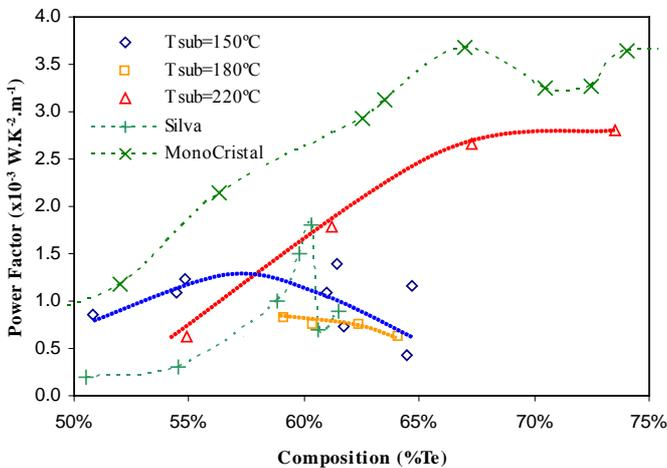
**Fig 6: Power factor of  $\text{Sb}_2\text{Te}_3$  as function of composition and substrate temperature. Results from literature [7] and from monocrystal [9] are also presented, for comparison.**
