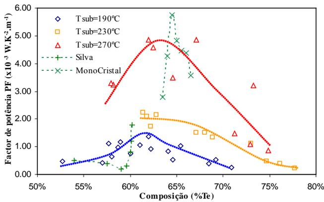
**Fig 5: Power factor of  $\text{Bi}_2\text{Te}_3$  films, as function of composition and substrate temperature. Results from literature [7] and from monocrystal [8] are also presented, for comparison.**
