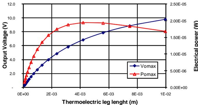
Fig 3: Open-circuit output voltage and power of a 1 cm<sup>2</sup> Bi<sub>2</sub>Te<sub>3</sub>-Sb<sub>2</sub>Te<sub>3</sub> thermoelectric generator, plotted as function of length of column.
