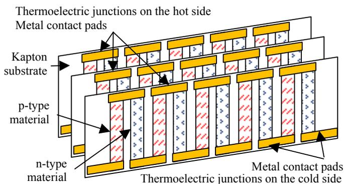
**Fig 9: Artwork of the proposed device. Foils with thermoelectric junction are stacked to obtain a large number of junctions. The last foil includes de Li battery and the charge-control circuit.**
