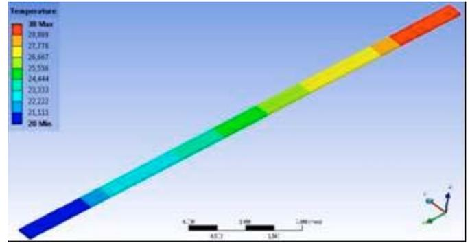
Fig 4: Temperature map of a thermoelectric pair in contact with body, obtained by FEM.
