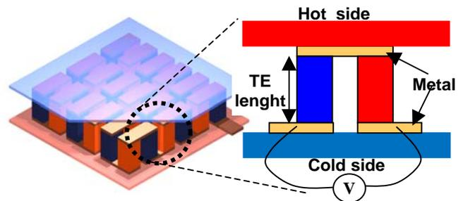
**Fig 1: Artwork of a thermoelectric generator.**
