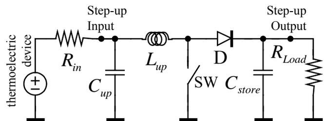
**Fig 8: Schematic of the step-up circuit.**
