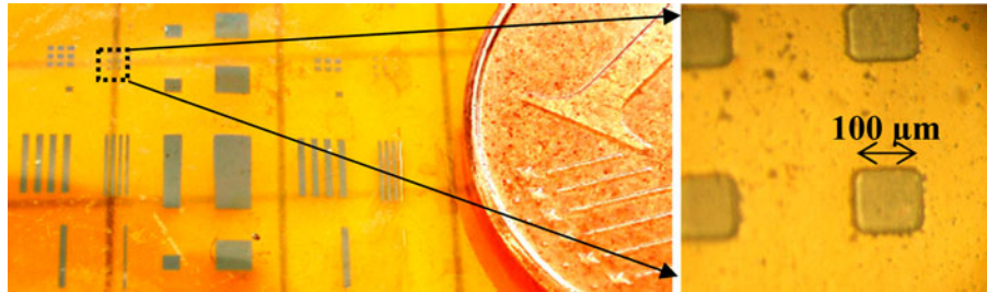
Fig. 6. Top view of test structures of thermoelectric films patterned by wet etching.
