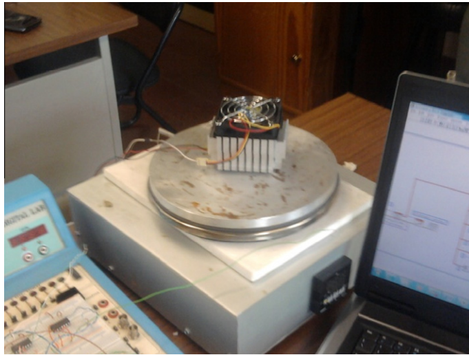
Fig. 2. The measurement setup showing a thermoelectric modules model TEC1-12707 between a controlled hot-plate and a controlled cooling fan. The personal computer running the LabView software connects to a data acquisition board model NI USB-6009 for controlling the heat flow (by way of the controlled hot-plate and the cooling fan) and for measure the produced currents and the respective voltages.
