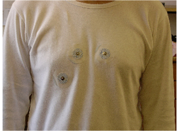
Fig. 8. A photo of the patient wearing a electronic shirt ready to plug the RF microsystem (antenna + transceiver). We can see the three connections for heart rate with a single electrode, respiratory function and posture.
