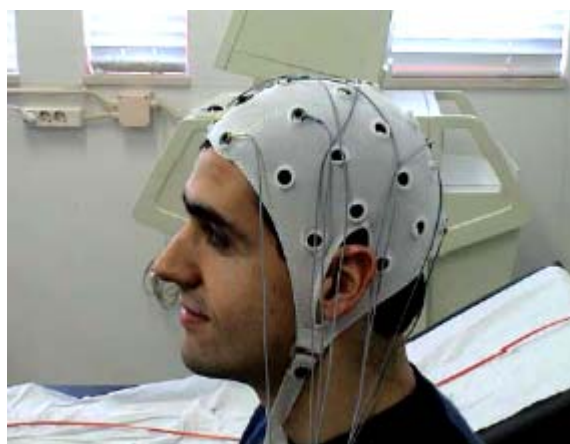
Figure 1. Classic EEG braincap with Ag/AgCl electrodes and respective wires.
