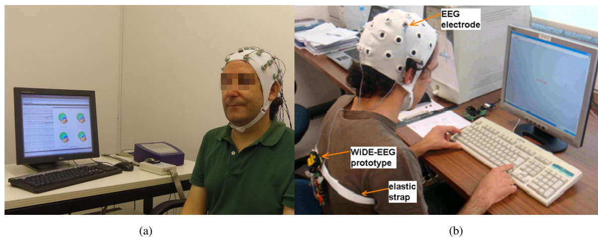
Figure 9: A subject (a) with a conventional EEG system based on wires and (b) with a wireless data acquisition, logging and transmission system prototype fixed with the help of an elastic band (the white strap) on the thorax region [51].
