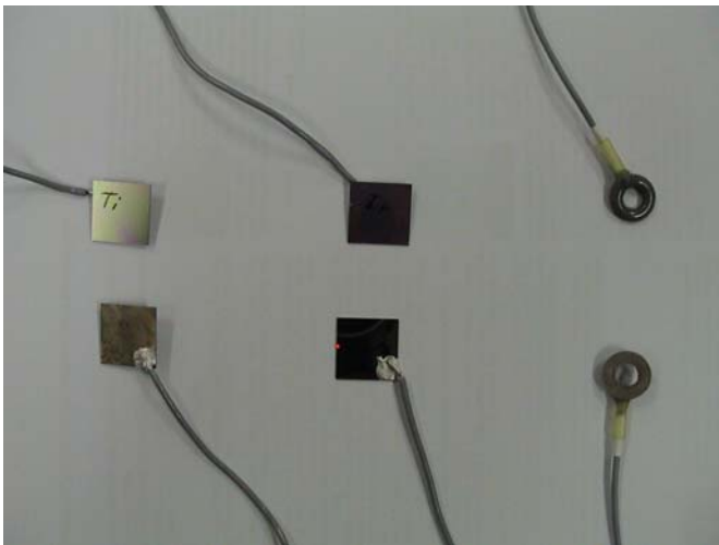
Figure 2. The fabricated/mounted electrodes in a set of pairs, from left to right: sputtered TiN electrodes, sputtered IrO 2 electrodes, and standard sintered Ag/AgCl ring electrodes.
