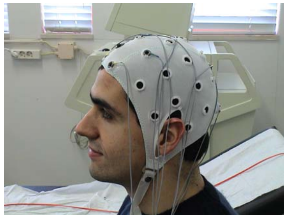
Figure 1. Classic EEG braincap with the electrodes distributed in the standard configuration 10-20 system.
