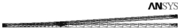
Figure 6: Non-stressed structure at white, non-bended lines. After applying pressure the structure bend and it is represented at blue.
