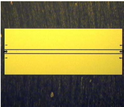
Figure 2: Photograph of the CPW cells used in substrate material characterization.
