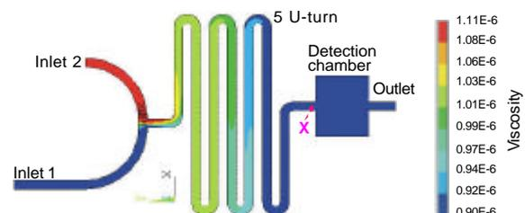
Fig. 3. Simulation flow of the diffusion mixing process. The graphic displays the viscosity profile of the model.
