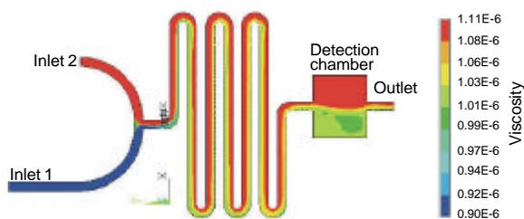
Fig. 5. Simulation results for 5 mg/dl uric acid concentration in urine.
