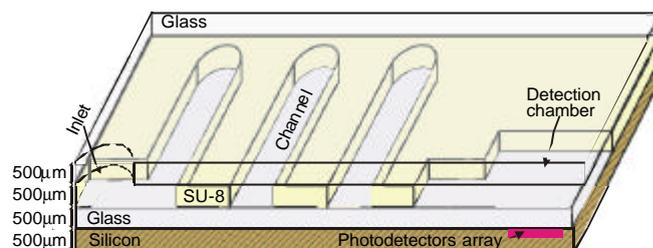
Fig. 6. Perspective cross-section drawing of the prototype integrated fluidic die.
