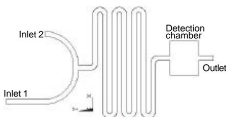
Fig. 2. Layout of the fluidic die (mixer).
