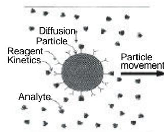
Fig. 1. Overview of the activities around the reagent-coated particle. The particle moves with a certain velocity through the sample while the immobilized reagent picks up analyte (governed by the kinetics).
