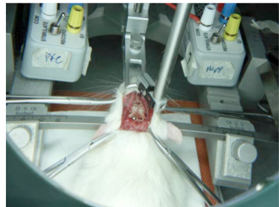
Figure 3 – Mechanical insertion tests on a male Wistar rat.
