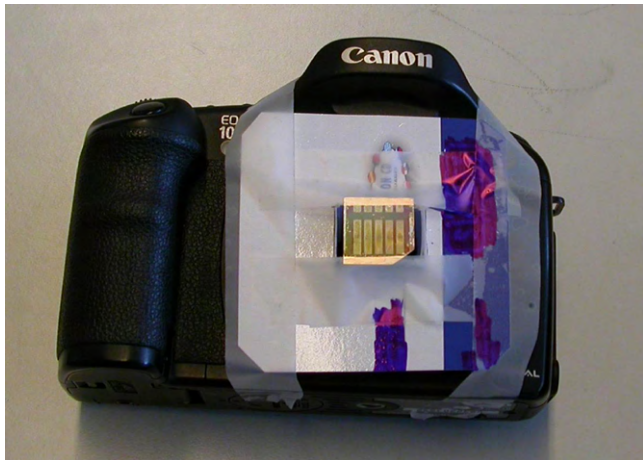
Fig. 9. LVOF deposited on the glass mounted at the entrance of the Camera. The glass contains five different LVOF filters.
