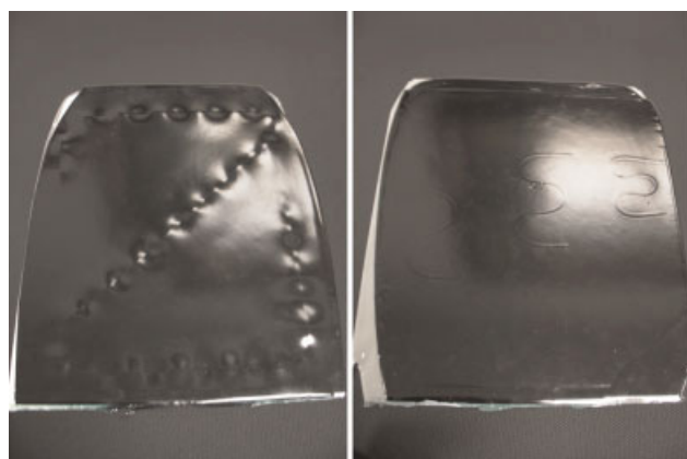
Figure 7. Prototype with fiber in straight line layout (left); Prototype with fiber in "S" layout (right). This figure is available in color online at wileyonlinelibrary.com/journal/pat .
