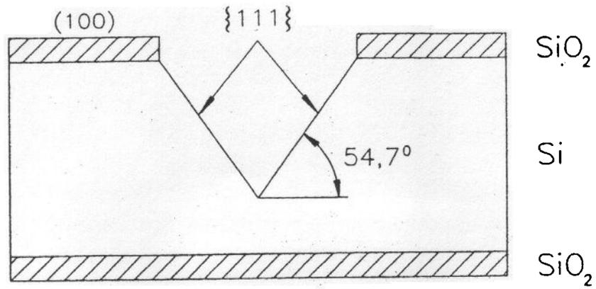
Fig. 2.7 Profile of an etched trench in (100)-silicon
