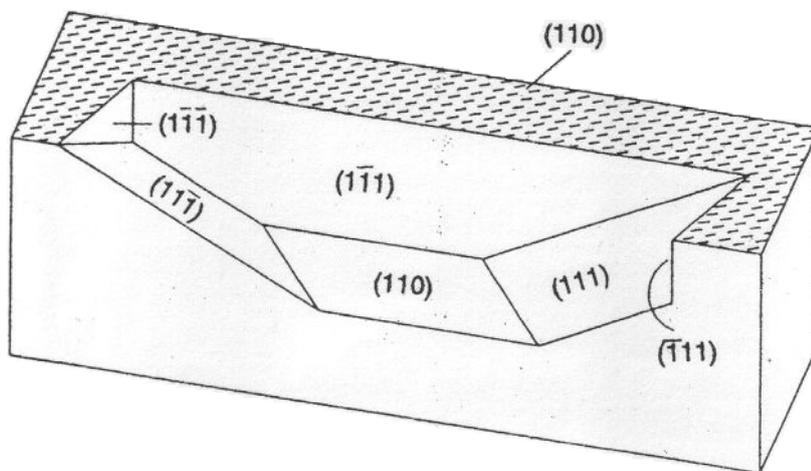
Fig. 2.9 Shapes of etched deepings in (110)-silicon
