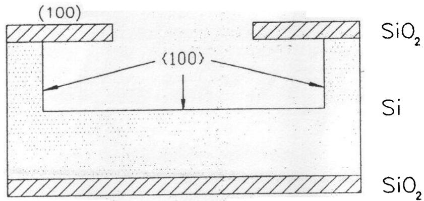
Fig. 2.8 Trenches with vertical walls in (100)-silicon
