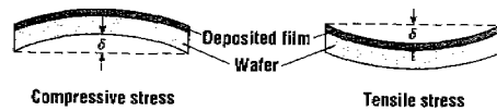
Figure 12.29 The change in wafer deflection may be used to measure the stress in a deposited layer. This is typically measured using a reflected laser beam.
