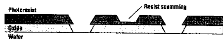
Figure 11.3 Resist scumming occurs when the photoresist is incompletely developed. The residual resist may serve as an etch mask to prevent a complete etch process.
