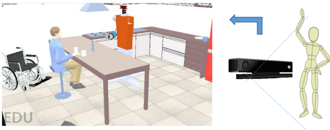
Figure 1: (Left) The virtual environment used in an assistive scenario. Work developed at the Mobile and Anthropomorphic Robotics Laboratory (MarLab). The robot ARoS helps an impaired person to have some refreshment. (Right) A Kinect 2 sensor.
