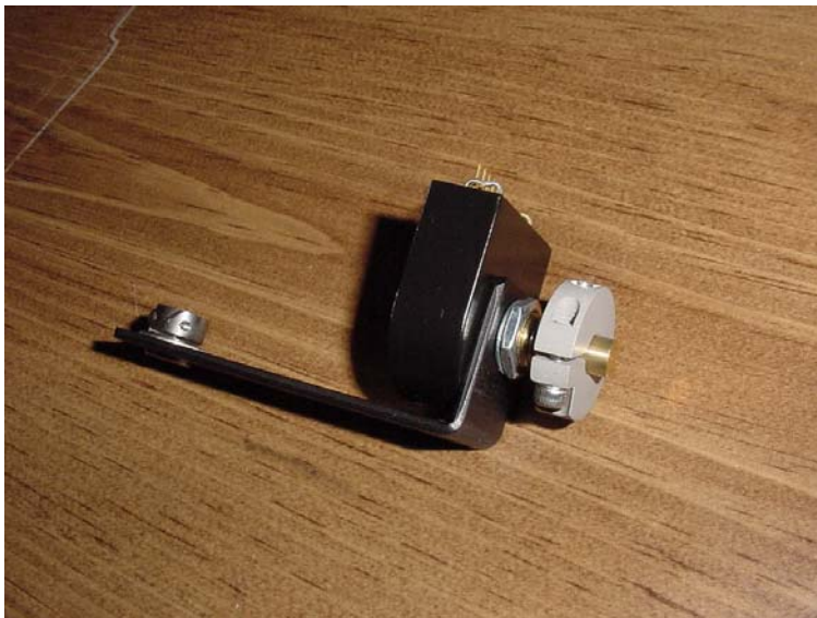
Figure 5-12: Furuta Link/Encoder Assembly
