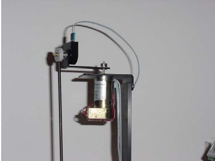
Figure 5-22: Furuta Pendulum Cable Routing
