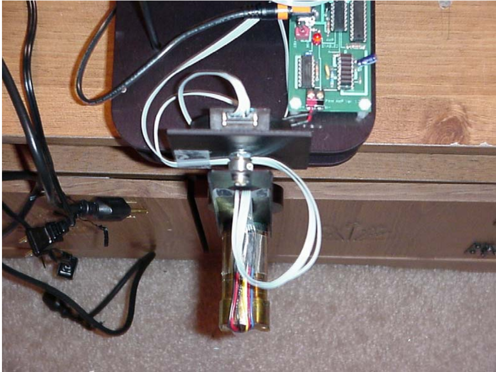
Figure 5-20 Reaction Wheel Cable Routing
