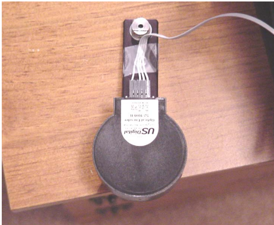
Figure 5-15: Taping the Encoder Cable to Pendubot Link-1
