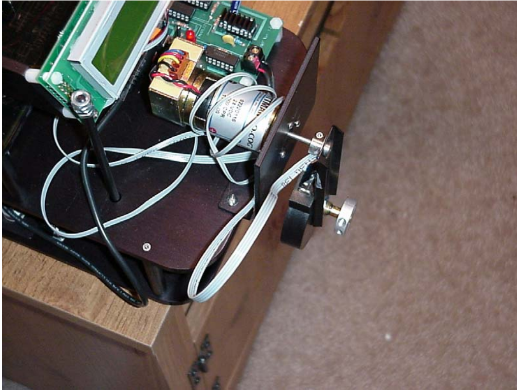
Figure 5-18 Pendubot Cable Routing
