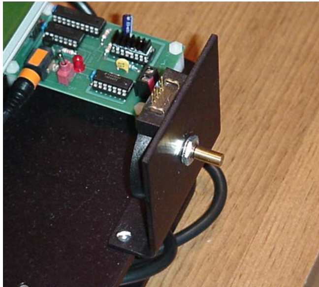
Figure 5-4: US Digital Encoder Attached to Front Bracket
