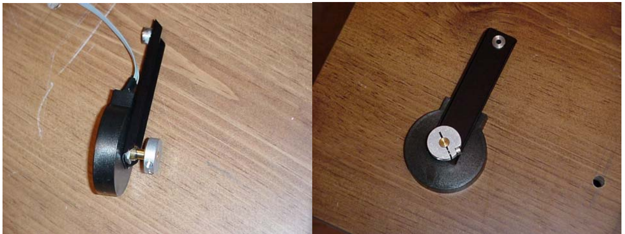
Figure 5-6: Pendubot Link/Encoder Assembly
