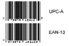
At first glance, the two barcodes look different. In UPC-A there is a number to the left and right of the barcode (a 0 number system and a 5 check digit), and below the barcode are two groups of 5 digits each (the manufacturer code and the product code). In the EAN-13 symbol, there is no check digit to the right of the barcode, and the numbers below the barcode consist of two groups of 6 digits each.
