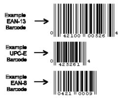
**NOTE**: The three barcodes above are shown only for relative size comparison. The three barcodes do *not* necessarily represent the same product, nor do they represent equivalent values. The similarities end there, however. Unlike UPC-E in which only 6 digits are explicitly encoded, EAN-13 explicitly encodes all eight digits; the parity of the digits carries no particular significance. This means that although EAN-13 is compatible with UPC-A, EAN-8 has absolutely no compatability with UPC-E.
